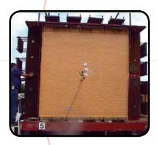
**Defend-X**<sup>®</sup> is a urethane-polyurea (type I) and polyurea (type III) base, two-component system. This high-tech system is spray-applied and cures as a rubber-like material. The material is used for blast and other protection systems.
